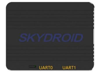
There are 2 serial ports on the air terminal, both with transmission function.
