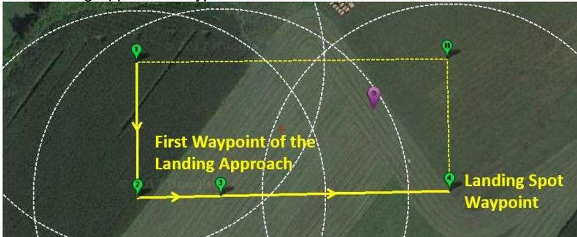
Note that waypoints 2, 3, and 4 are lined up. This makes it easier for the autopilot to keep the plane on the approach track as the landing algorithm limits the bank angle when the plane is close to the ground.
