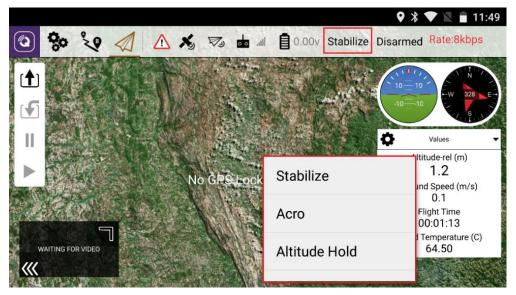
3. When selecting "Values" option, joystick will also malfunction. Thus, please do not frequently switching among different options or keep the menu open. If it is necessary to switch during the flight, make it as fast as possible.
