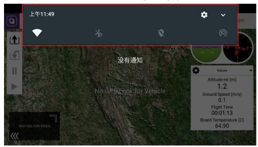
2. When selecting flight mode on Herelink QGC, a window will be popped up. Stay focus on the pop-up window will also cause joystick malfunctioning. Therefore, it is better to use buttons (via hardware) instead of touch screen (via software) to switch flight mode during the flight.
