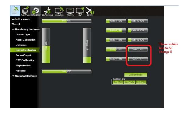
We have non used channels with low values... (rc15\_Trim and rc16\_trim and maby rc13 \_trim as well)
