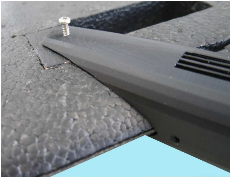
Fix the motor carrier with 2 screws on the back on top and below the wing via a piece of plywood
